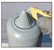
Insert a utility knife in the top cone, cut down to feel the inside edge of the pipe. Use the inside edge as a guide to carefully cut out and remove the cone.
