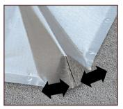
If pitch adjustment is needed, push the flange hips in to incease pitch, pull the flange hips out to decrease the pitch.
